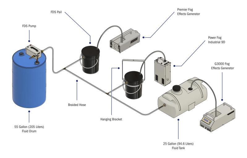
Note: The Fluid Distribution System (FDS) can also be configured for use with the Bubble Master and the Silent Storm Snow Machine. The FDS can only be used with industrial option machines.
