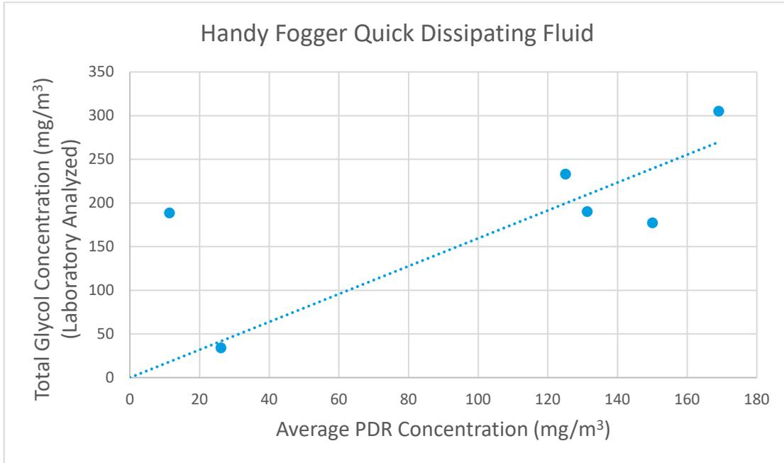
**Figure 2.** Calibration curve for Ultratec’s Handy Fogger with Quick Dissipating Fog Fluid, based on glycol laboratory data. Calibration factors, based on slope of curve, are 1.60 (mg/m<sup>3</sup> glycol) / (mg/m<sup>3</sup> aerosol).
