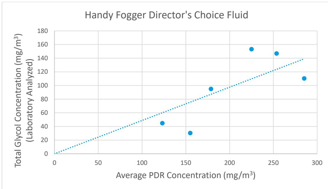
**Figure 1.** Calibration curve for Ultratec’s Handy Fogger with Director’s Choice Fog Fluid, based on glycol laboratory data. Calibration factors, based on slope of curve, are 0.49 (mg/m<sup>3</sup> glycol) / (mg/m<sup>3</sup> aerosol).
