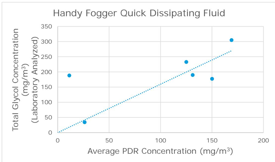
**Figure 5:** Calibration curve for Ultratec’s Handy Fogger with Quick Dissipating Fog Fluid. Calibration factor, based on slope of curve, is 1.60 (mg/m<sup>3</sup> glycol)/ (mg/m<sup>3</sup> aerosol).
