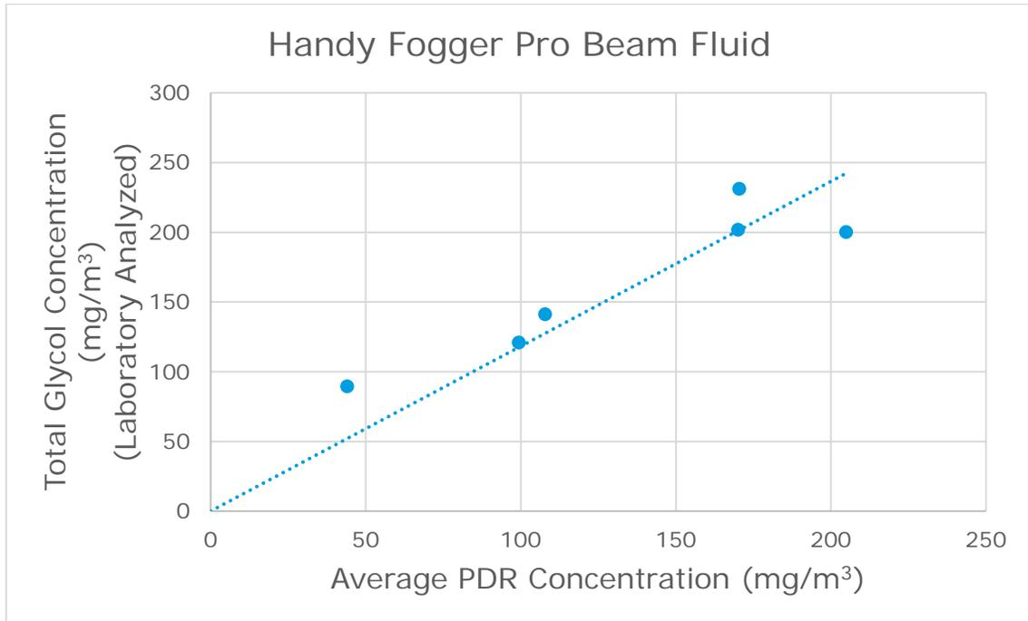
**Figure 3:** Calibration curve for Ultratec's Handy Fogger with Pro Beam Fog Fluid. Calibration factor, based on slope of curve, is  $1.18 \text{ (mg/m}^3 \text{ glycol) / (mg/m}^3 \text{ aerosol)}$ .
