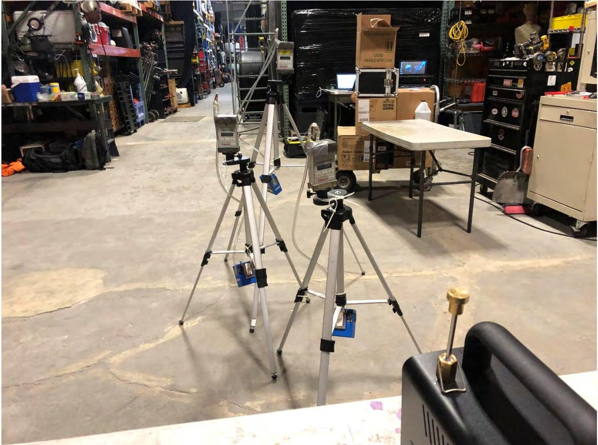
**Figure 1.** Configuration for calibration factor procedure, consisting of the tripod assemblies with sampling pumps, OVS tubes, and aerosol monitors.
