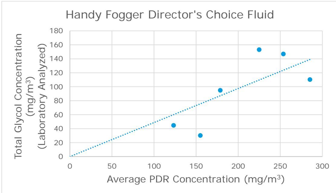
**Figure 4:** Calibration curve for Ultratec’s Handy Fogger with Director’s Choice Fog Fluid. Calibration factor, based on slope of curve, is 0.49 (mg/m<sup>3</sup> glycol)/ (mg/m<sup>3</sup> aerosol).
