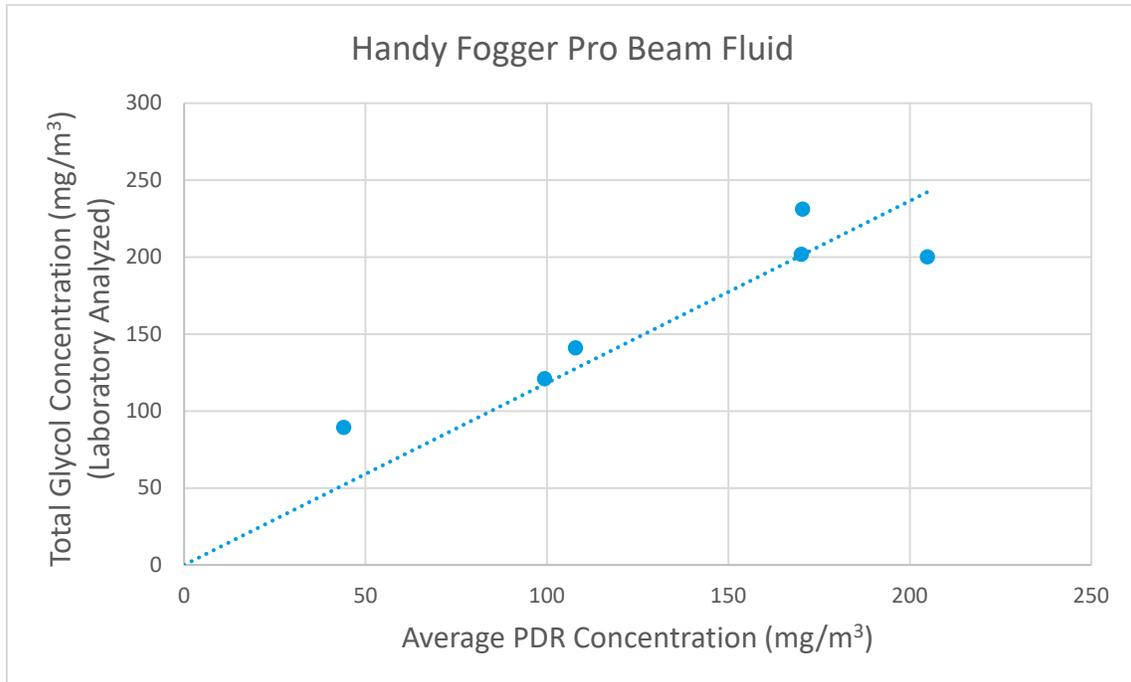
**Figure 3.** Calibration curve for Ultratec’s Handy Fogger with Pro Beam Fog Fluid, based on glycol laboratory data. Calibration factors, based on slope of curve, are 1.18 (mg/m<sup>3</sup> glycol) / (mg/m<sup>3</sup> aerosol).
